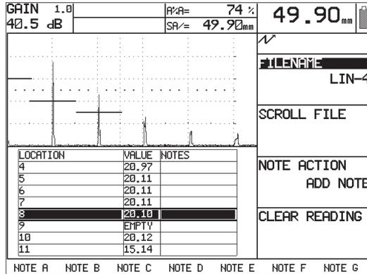
The status and, if necessary, the saved notes are displayed for all measurement locations of the file. The following displays are possible for the status of a location:
