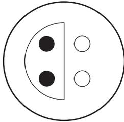
View of the 4-pin power supply socket
