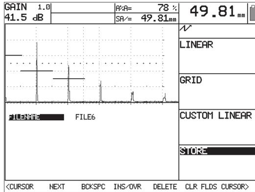
The Data Logger enables you to define different test jobs. To do this, you have to select a corresponding file type for the Data Logger. The following options are available:
