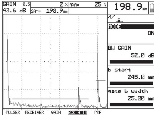
The echoes in gate B are now shown with a different gain from that of the echoes in the rest of the test range. You can read the gain for the test range in the gain box. The gain for gate B is indicated in the function **BW GAIN**.
